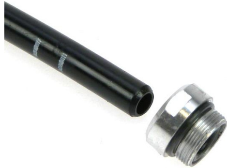
Fig. 22: Bushing pulled off the tube
