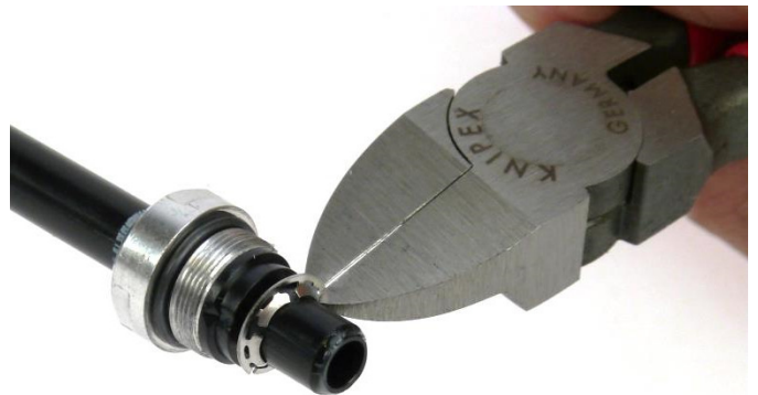
Fig. 19: Cutting the grip disc
