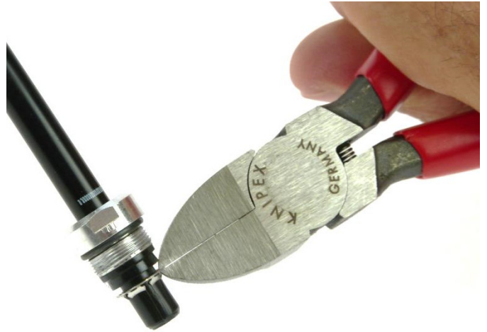
Fig. 19: Cutting the grip disc
