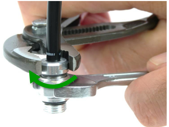
Fig. 17: Screwing the sealing set out of the male fitting
